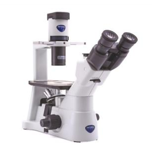
Inverted trinocular brightfield/phase contrast microscope, IOS
